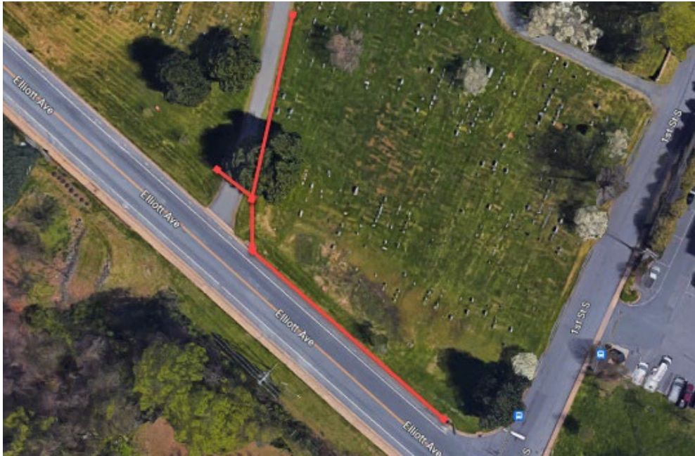
Figure 18 – Map showing four known storm sewer pipes (red lines) in within the study area.
