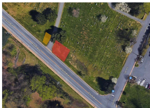
Figure 9 – 2023 GPR Scanning associated with this study. Orange shade is successful scanning area. Red shade is unsuccessful scanning area due to soil saturation.
