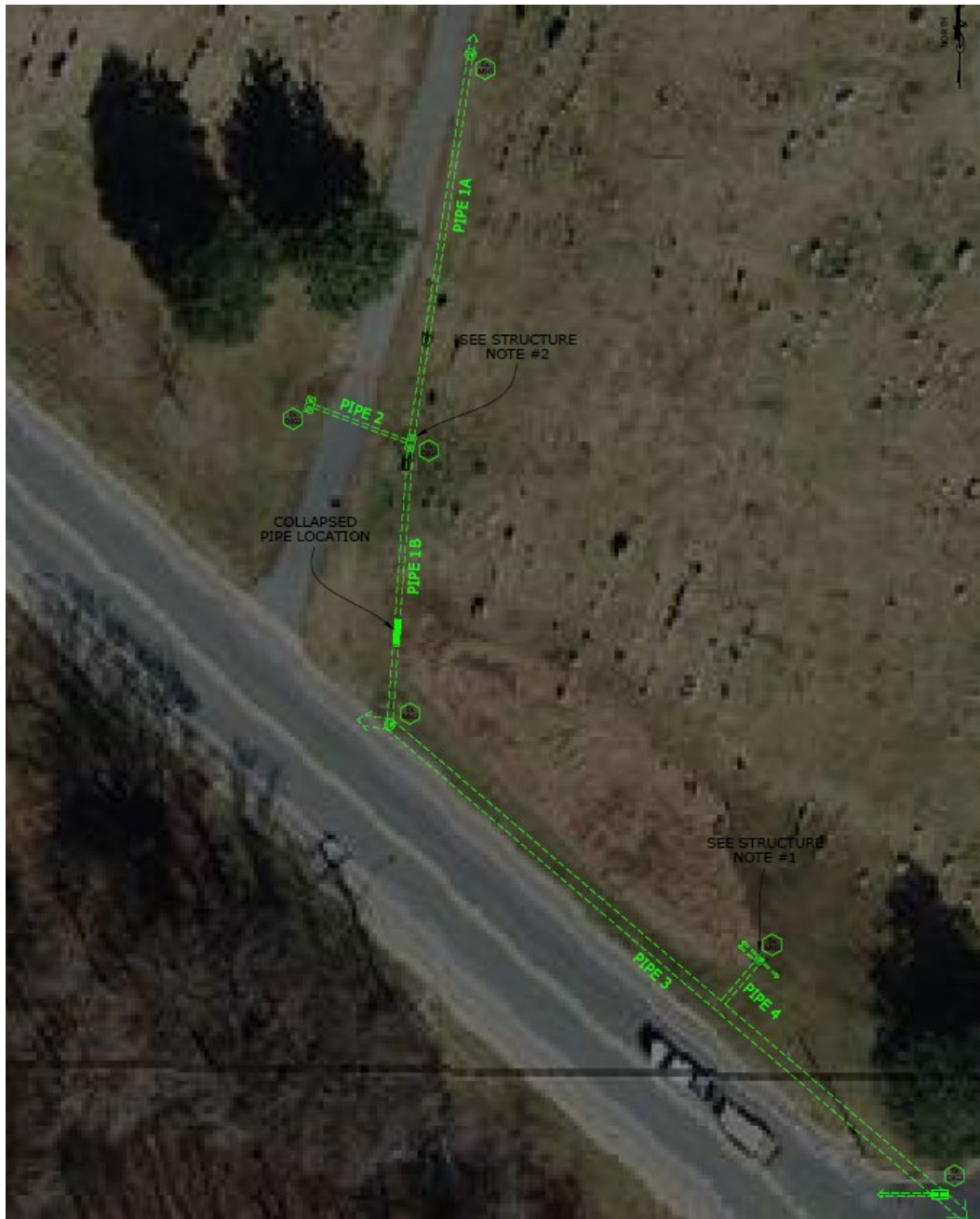
Figure 25 - Note the Location of the broken pipe, and the variation of the ground cover color between the broken pipe and the grounds adjacent to the pipe.
