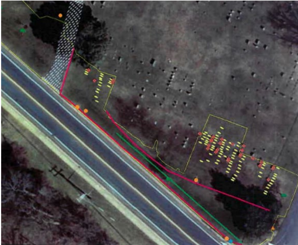
Figure 7 – Plan showing location of buried utilities (red and green lines), and grave like anomalies (yellow) and grave markers (red). The thin yellow outline represents the study area. NAEVA Geophysics, Inc., 2017.
