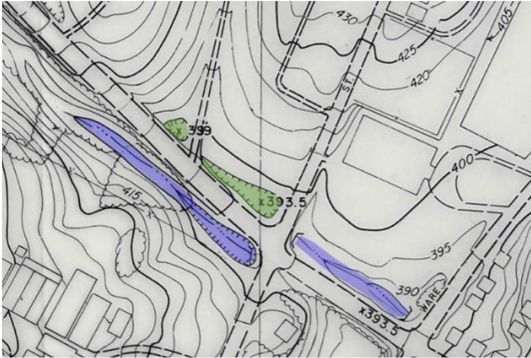
Figure 17 – A topographic map showing the vicinity of Oakwood Cemetery and the location of what remains of the natural tributary low-lying areas (blue shade). Also note the low-lying formed to the north of Elliott Avenue and they are specifically demarcated by a different line-type in the survey (green shade).
